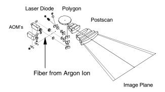
Figure 1. Laser Recorder Unit of Agfa Digital Minilab
